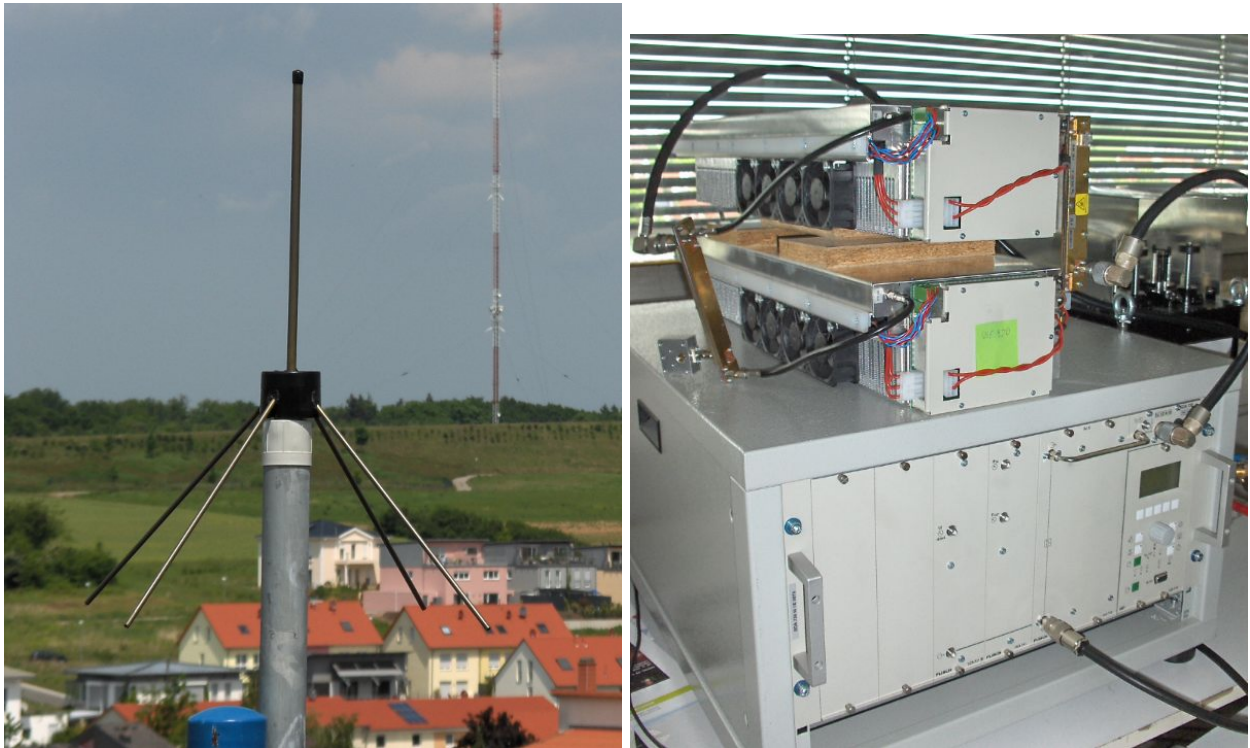
Fig. 3.3: Left: Self-made groundplane antenna of TX FH (foreground), watching over to TX RB (background); Right: Power amplifier and filter installation of TX FH using Plisch-equipment for the radiation of 180 W.
